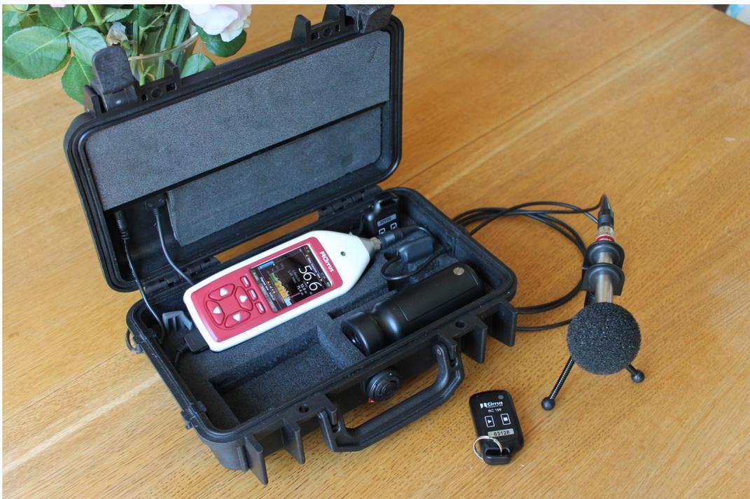
The sound level meter runs all the time recording parameters such as the periodic Leq (average sound level), statistical parameters that describe the background noise levels and the level every second, to provide a graph of the sound level over time.
